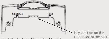
Do not insert anything other than the specially designed key into this slot.
