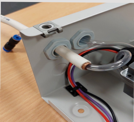
The images above depict the copper pipe that leads from the Pressure Sensor, contained within the white port enclosure.
