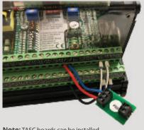
**Note:** TASC boards can be installed locally into the OS2 Shevtec controller
