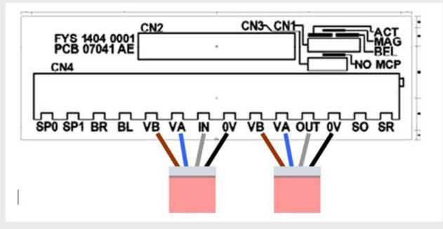
Ensure a consistent colour scheme is used all around the loop
