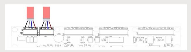
Ensure a consistent colour scheme is used all around the loop
