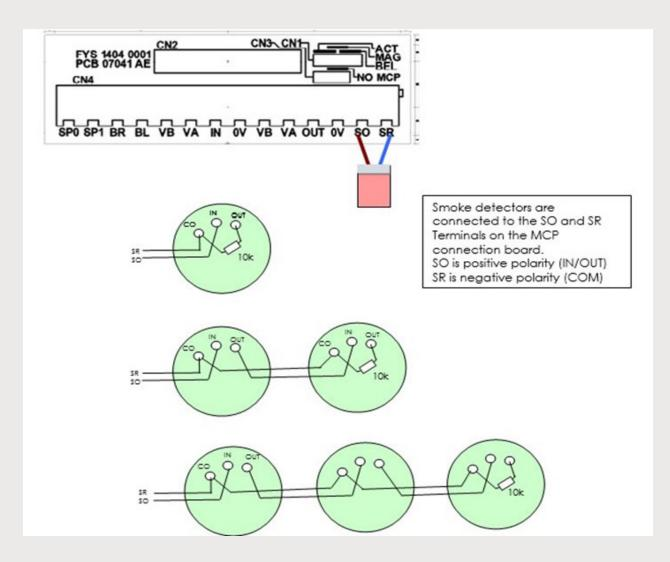
The illustration above shows S.E.Controls preferred timesaver bases - Connection to other makes of smoke detectors will be similar.
