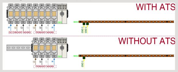
**Important:** The Mains Switch Disconnector will not isolate the circuits linked to connectors X28, X29, X30 and X32. These terminals are used to link the panel to external parts of the system. To isolate that part of the circuit, please check the devices to which they are linked. These terminals are connected to internal components via orange cables, which should help to identify which parts of the panel may remain energised even when the Mains Switch Disconnector is in its OFF position.
