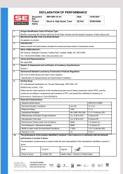
The Declaration of Performance (DoP) and the product certification mark are the ultimate proof of compliance which illustrates the vent profile and actuator have been tested together as a single solution to all declarable essential characteristics of EN12101-2:2003.
