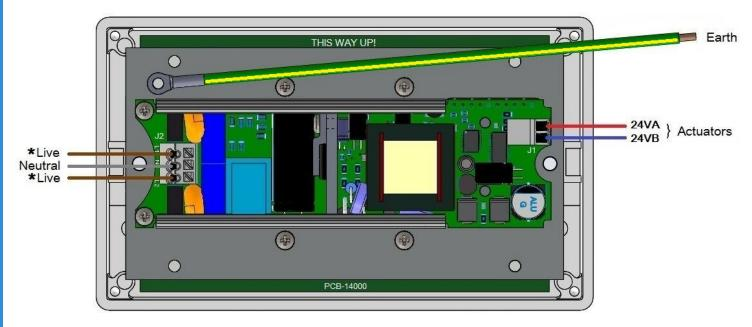
\*Live can be connected to either L1 or L2 inputs
