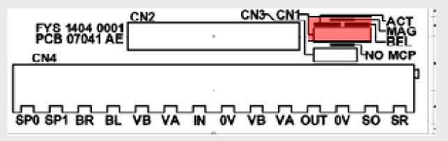
The actuators mode jumper on each connection board must be set at every MCP to match the type of actuator. This jumper has 3 positions.
