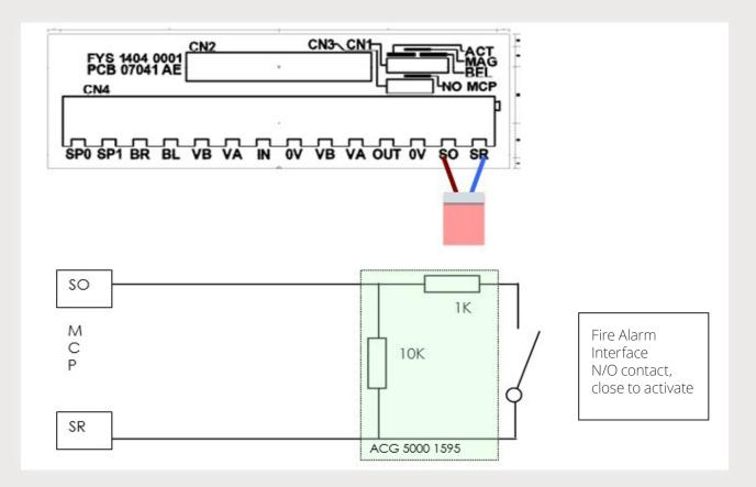
The contact monitoring module should be installed as close to the fire alarm interface as possible (commonly inside the same enclosure), to allow monitoring of the full length of the cable to the MCP.
