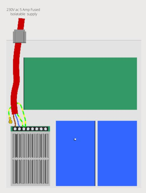
The power supply earth terminal also connects to the chassis - ensure this earth connection is properly made.
