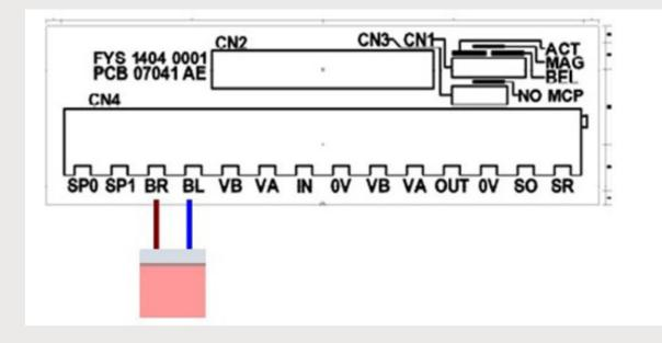
The actuators are connected to the BR and BL terminals on the MCP connection board.
