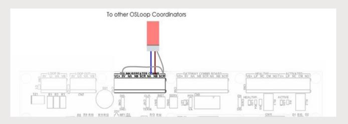
Coordinator to coordinator connections do not require power, and may be wired in two core plus earth. In this case, connect the protective screen to 0V at both ends.
